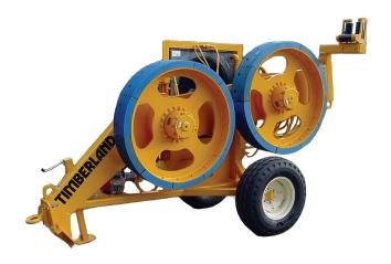
The T40-1H/1DD is suitable for tensioning single conductor with infinitely variable tensioning control of the conductor.
